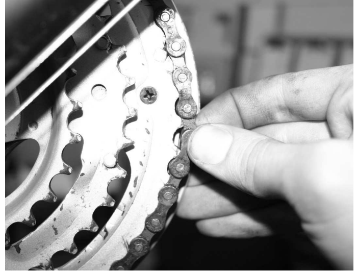
Part-worn, but probably still OK to replace the chain
