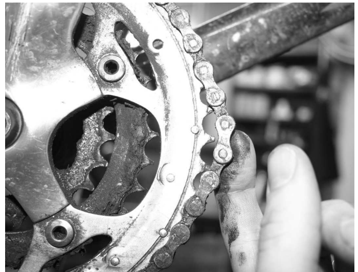
Worn out: drivetrain is slipping and must be replaced
