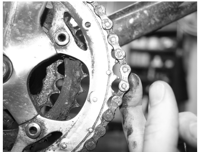
Worn out: drivetrain is slipping and must be replaced
